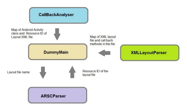
Figure 26: Identifying Android call back methods from XML Layout file
