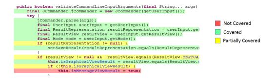
Figure 33: Color code displaying the coverage in Java source editor
