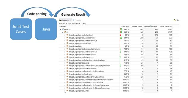
Figure 32: Code Coverage displayed in Coverage window
